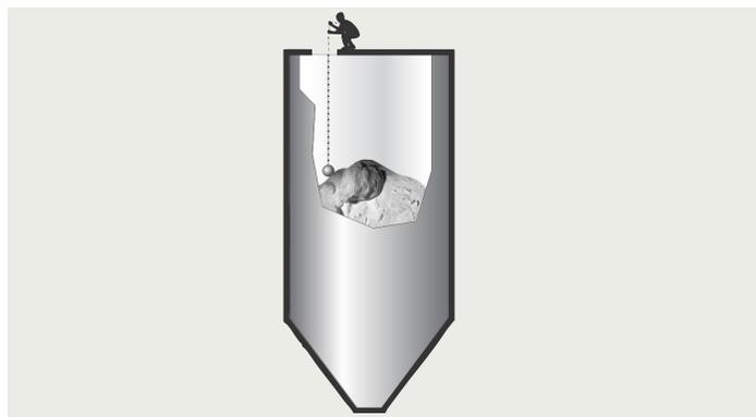
Manual measurement with rope and weight
