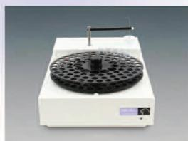
The AA100 carousel sampler is robust and simple to use. Samples can be added at any time during the run.
