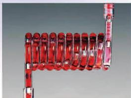
The chemistry manifold is comprised of close-tolerance glass components, which are chemically inert and allow for easy visual check of operation.
