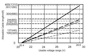
Cable cross section area: 1.25 mm<sup>2</sup> (1100 mm or larger, power consumption 32 W)
