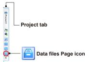
The data files in the data file save destination directory are listed. Only data files saved in binary format are displayed. Data files saved in Excel format are excluded.
