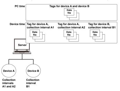
The device number, device name, and device acquisition interval are included in the names of data files. Below is the file name format when date and time are included. FileName-DeviceNo-DeviceName-Interval-YYYYMMDDhhmmss.ext FileName: The file name string specified by the user DeviceNo: Device number on the Device Setting Page DeviceName: Device name on the Device Setting Page Interval: The acquisition interval of each device
