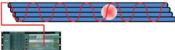
DTSX can be easily deployed along cable tunnels, ducts, trays or rack systems where heat build-up could indicate the potential for a fire hazard, or conductor over-temperature condition.
