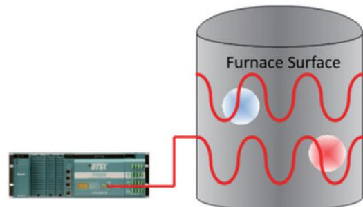
Furnace chamber or reactor vessel liner deterioration diagnosis via external wall surface temperature profiling.
