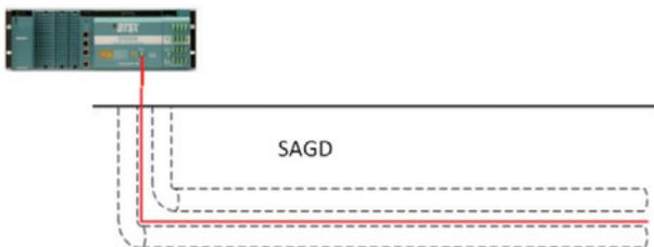
Wellbore temperature distribution profile can be used to detect thermal events related to steam breakthrough and oil & gas intake position, or other geophysical conditions.
