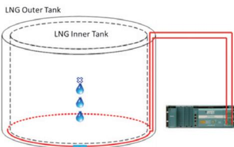
DTSX is commonly used for LNG tank leak detection by monitoring the expected differential in temperatures between the inner and outer liners comprising the tank system.
