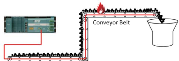
DTSX can be used to detect heat build-up along conveyor systems indicating mechanical component failure or potential combustion conditions.
