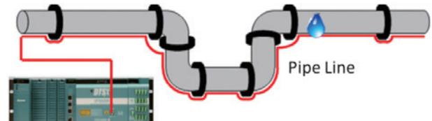
DTSX thermal profiles can be used to detect leak locations along LNG, liquid ammonia and other compressed gas pipelines where escaping content creates a thermal variance from normal background temperatures.
