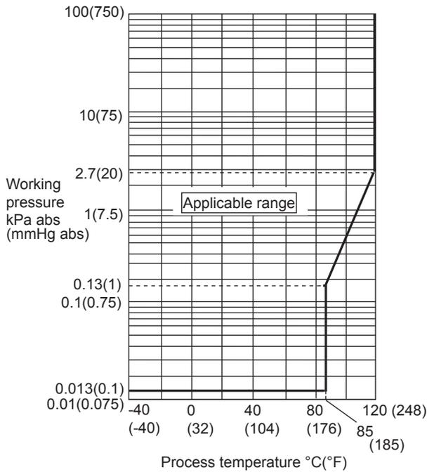
**Figure 1-1. Working Pressure and Process Temperature [For EJA510E]**
