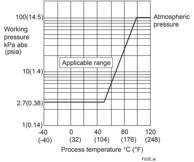
**Figure 1-2. Working Pressure and Process Temperature [For EJA530E]**
