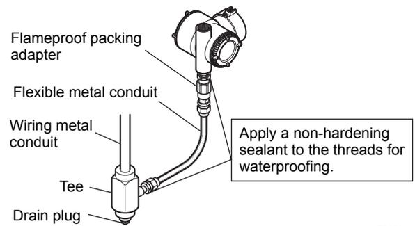
Figure 6.14 Typical Cable Wiring Using Flameproof Packing Adapter
