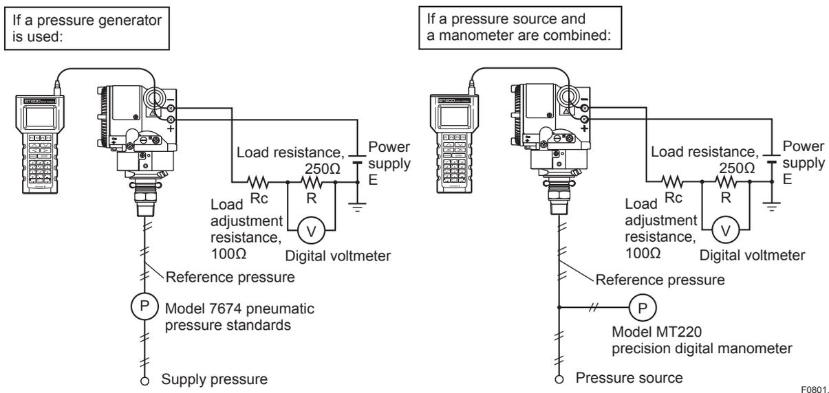
**Figure 8.1 Instrument Connections (4 to 20 mA output)**
