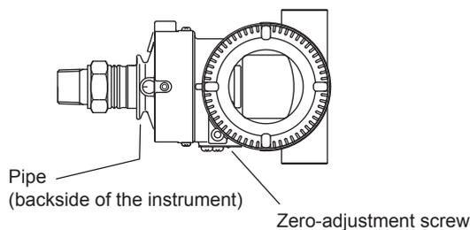
If the zero-adjustment screw is positioned other than downwards after installation, rotate the housing until it is positioned downwards.
