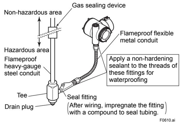
Figure 6.15 Typical Wiring Using Flameproof Metal Conduit
