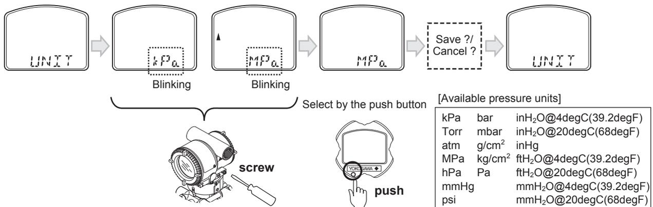
In addition to the above units, mmAq@4degC, mmAq@20degC, mmWG@4degC and mmWG@20degC are available for BRAIN communication type.
