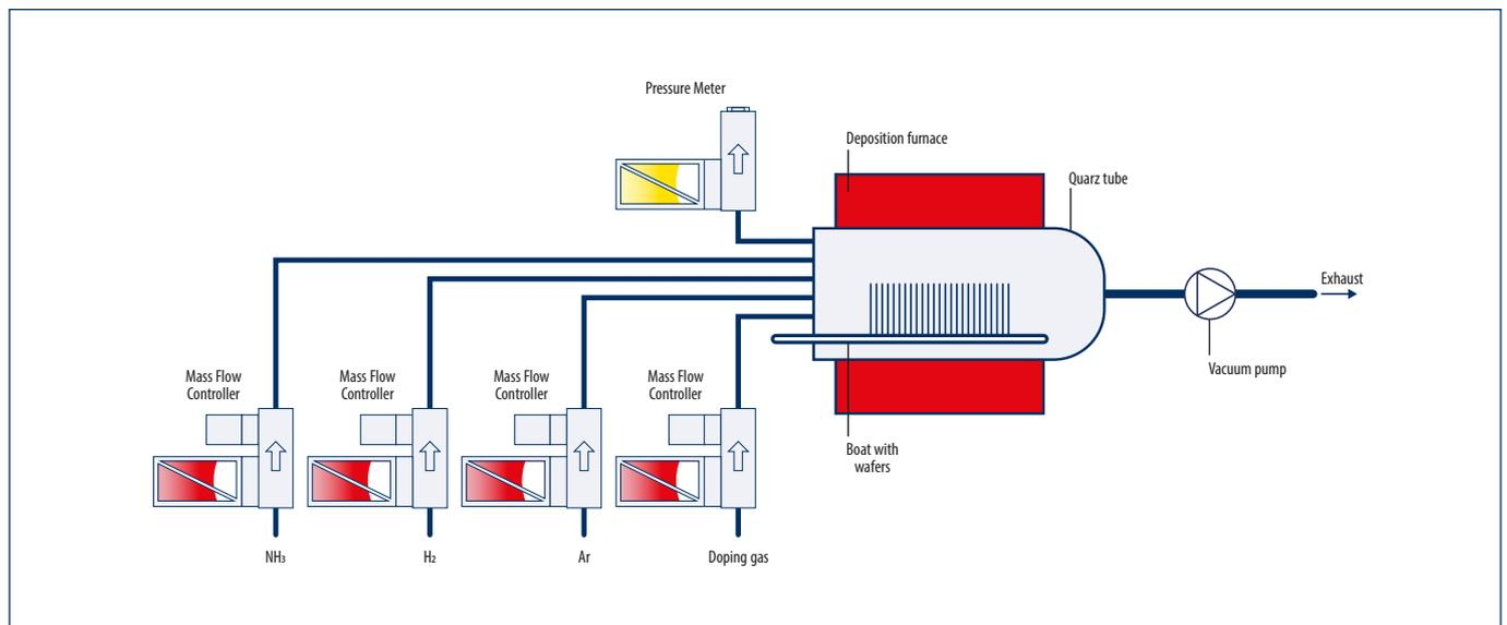
Schematic drawing of a Chemical Vapour Deposition process
