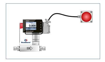
EL-FLOW Prestige instruments offer alarm and counter functions as a standard feature. To reset the counter value, e.g. locally displayed by a BRIGHT R/C-module, the user should operate the push-buttons. Alternatively, using the digital input option of the programmable pin 5, an external input signal can be sent to the instrument to reset the counter.
