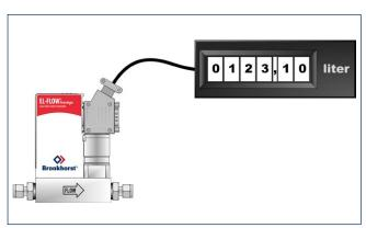
The programmable pin 5 (9-pin sub-D connector) can be set for a pulse output per quantity, as defined by the user. This pulse can be fed directly to remote totalizing counters, digital readout devices or control instrumentation.
