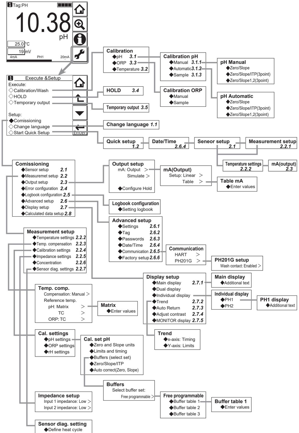
Figure 1.1 Menu structure of pH/ORP (the number after the item refers to the relevant section)
