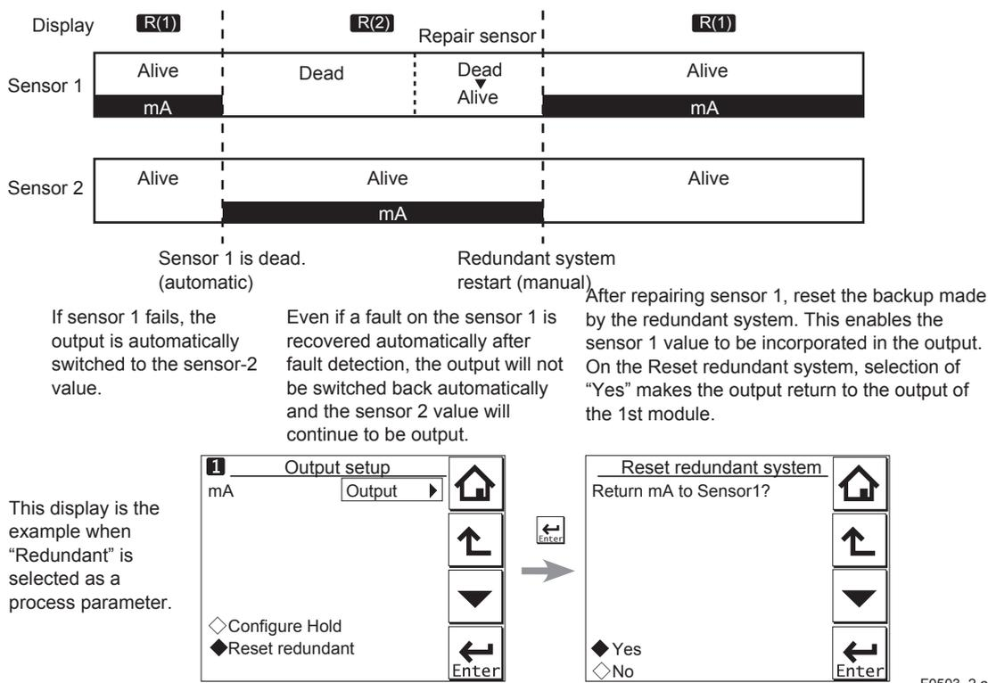
**Figure 2.4 Redundant system**
