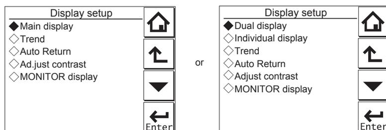
Figure 2.7 Display setup screens for a single module (left) and two modules (right)
