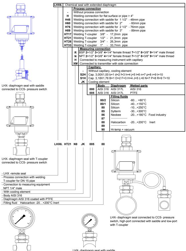
LHX- diaphragm seal with T-coupler connected to pressure gauge
