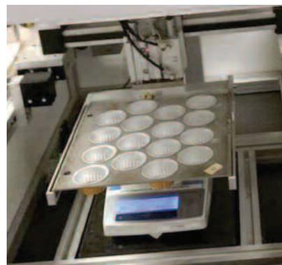
Weighing of samples before drying to assess dryness or after ashing can be done with SEAL robotic systems or inline with various other steps on our MiniLab robotic system.
