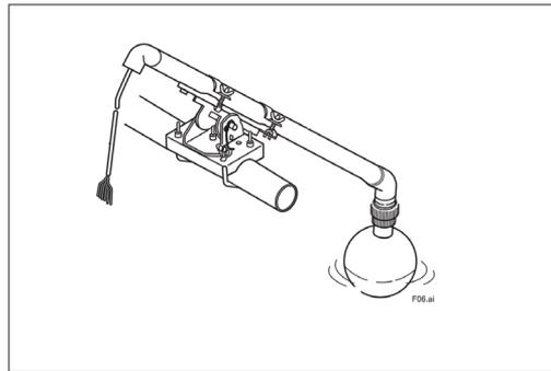
**Fig. 3:** PB350G/PB30 angled floating ball holder
