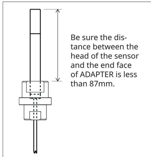
**Fig. 10:** Sensor positioning
