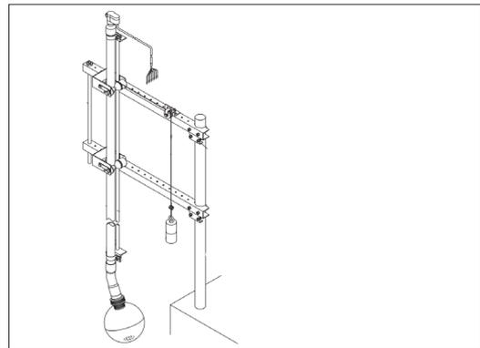
**Fig. 4:** PB360G vertical floating ball holder
