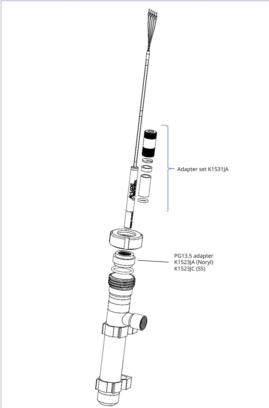
**Figure 12.** DO71 installation in Yokogawa FF40 fitting<sup>6</sup> using the adapter K1531JA sensor adapter set to fit in PG13.5 fitting adapter K1523JA (Noryl) K1523JC (SS)
