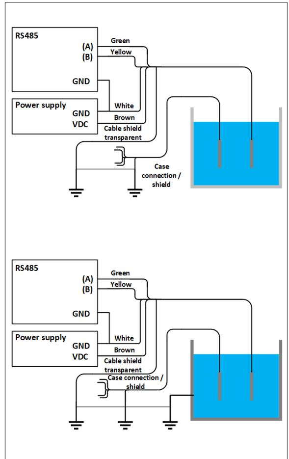
**Fig. 15** Example grounding DO71 when installed in a GLASS/PLASTIC (top) and METAL TANK (bottom)
