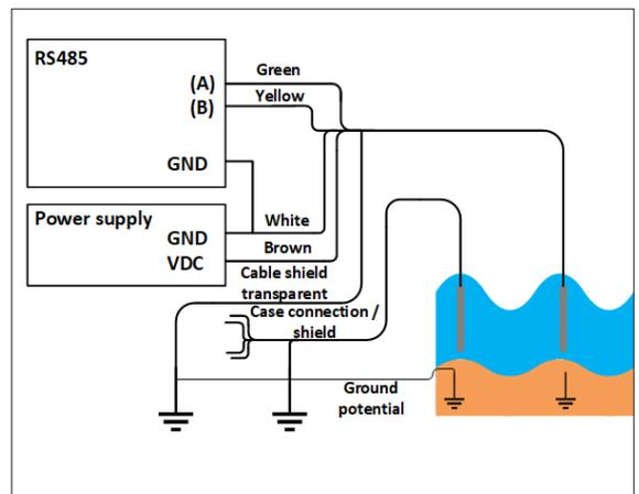
**Fig. 16:** Example grounding DO71 when installed in OPEN WATER
