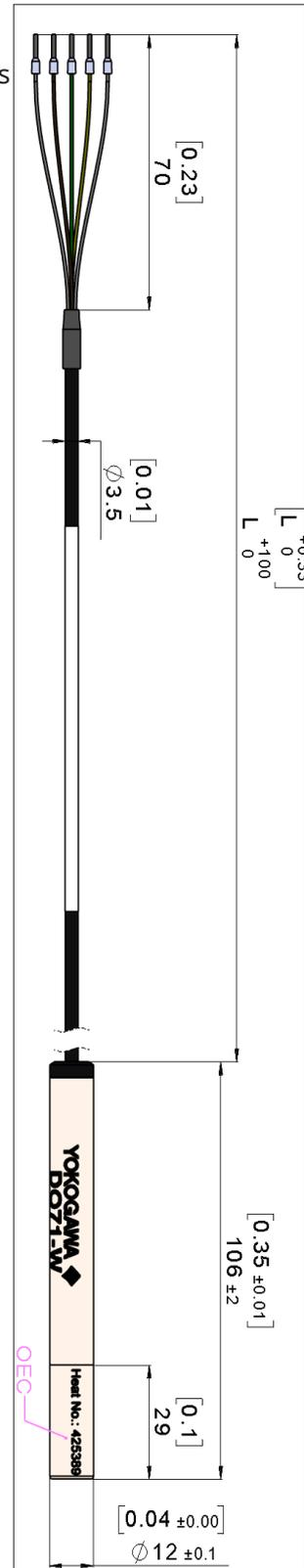
**Fig. 13.** Dimensions DO71 in mm [inches]
