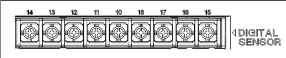
**Fig. 14.** D6 module terminal assignment for DO71 dissolved oxygen sensor
