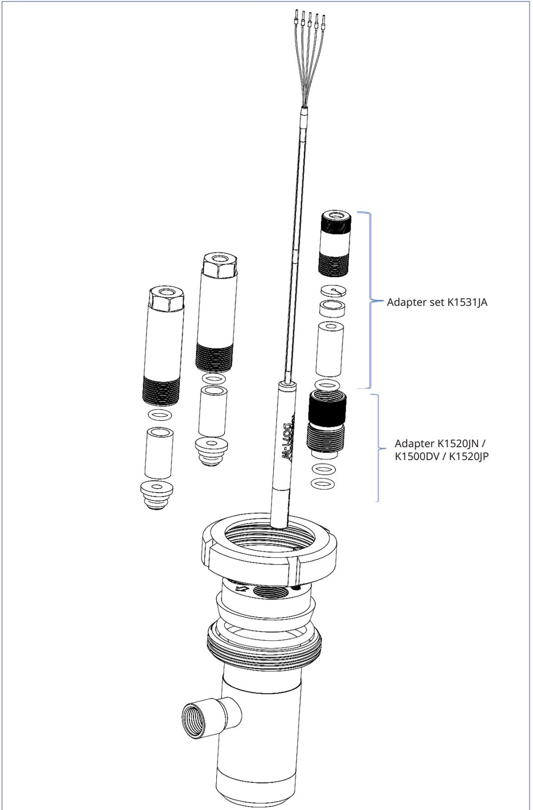
**Figure 11.** DO71 installation in Yokogawa FF20 fitting<sup>6</sup> using the adapter K1531JA sensor adapter set and adapter to fitting K1520JN, K1500DV or K1520JP
