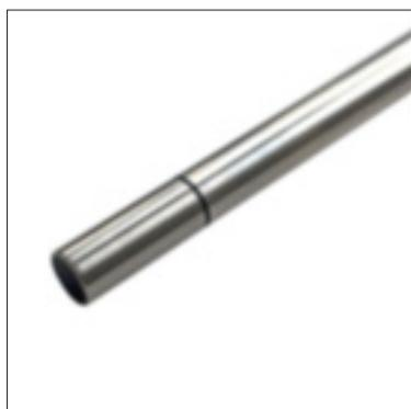
**Fig. 15:** O-ring visible - wrong OEC installation
