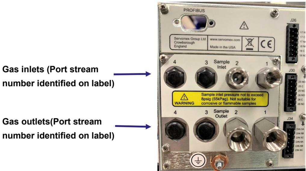
**Figure 3-1: Gas inlets and outlets on rear of the analyzer**
