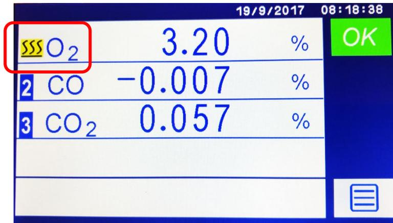
Figure 3-10: Home screen for a 3-transducer analyzer showing the O<sub>2</sub> warming up
