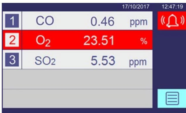
Figure 4-9: Home screen (3 transducer analyzer), showing O<sub>2</sub> alarm
