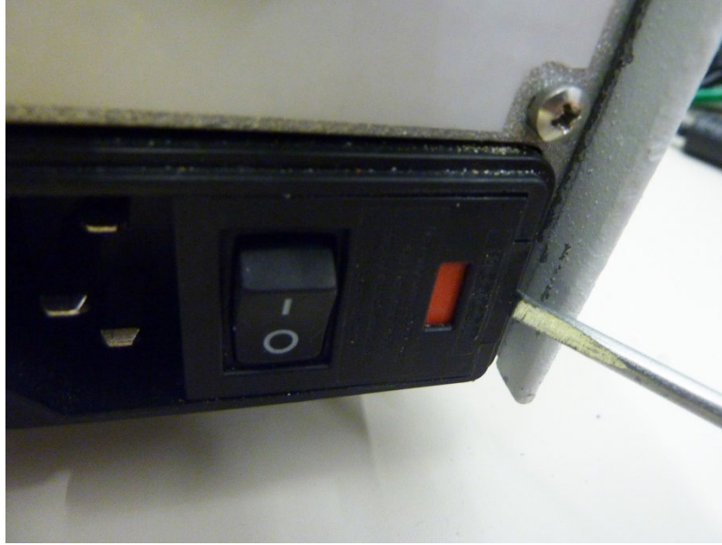
Figure 8-1: Open the fuse panel
