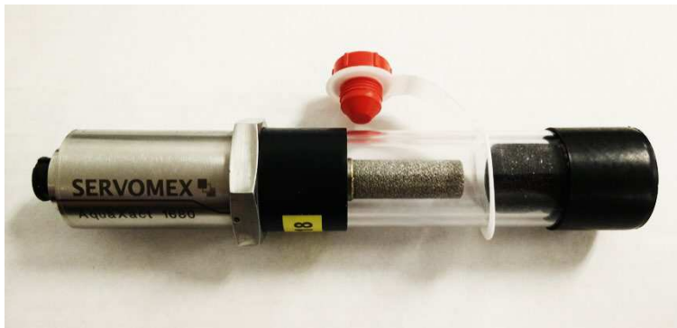
Figure J-8: AquaXact 1688 Al 2 O 3 transducer glass storage bottle
