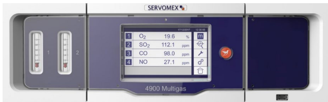
Figure 4-5: Gas Flow Meter location on front panel of the standard analyzer
