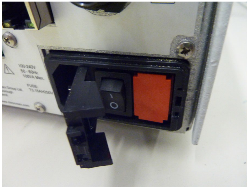
Figure 8-2: Fuse panel opened
