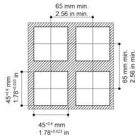
Dimensions: 48 x 48, depth 62 mm (depth from the panel surface) (1.89 x 1.89 x 2.87 in.)
