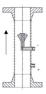
Liquid Vertical Flow Upwards Type CT
