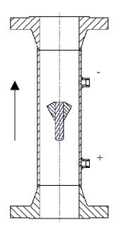
Gas Vertical Flow Upwards Type WT
