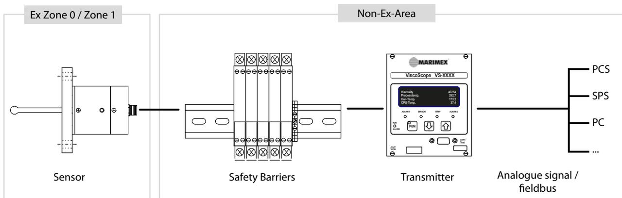
Typical system design for installation in Ex-Area
