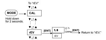
Figure 6.13 Display Software Revision "rEV"
