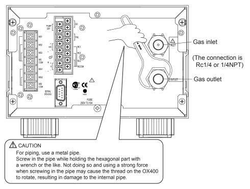
Figure 4.2 Piping for Sample Gas
