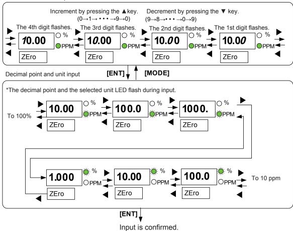
Figure 6.21 Example of Operation to Input Numerical Value, Decimal Point, and Unit
