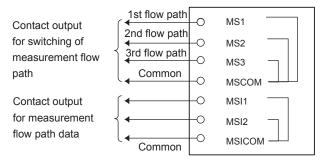
Figure 4.3 External Wiring Diagram
