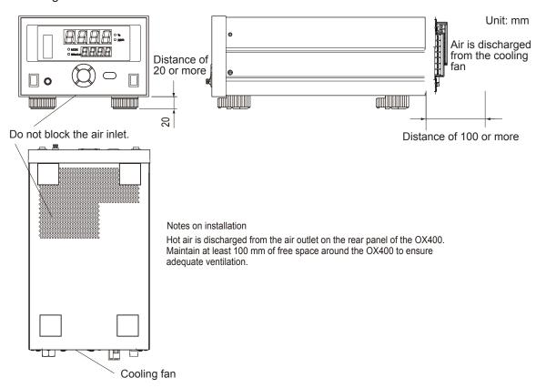
Figure 3.1 Notes on Installing Desktop Type
