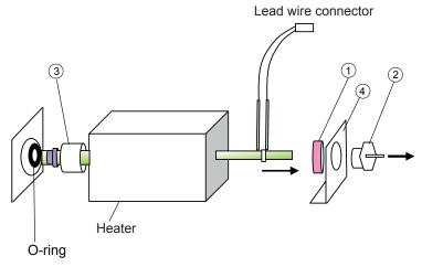
Figure 7.2 Removing Sensor
