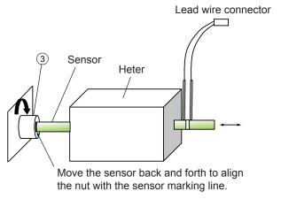
Figure 7.3 Installing Sensor
