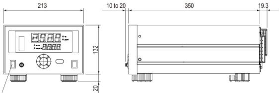
Note: Pump ON/OFF switch; when no suction device [-N] is specified for the sampling method, this switch is not installed.
