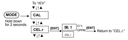
Figure 6.12 Displaying Cell Resistance Value "CEL.r"
