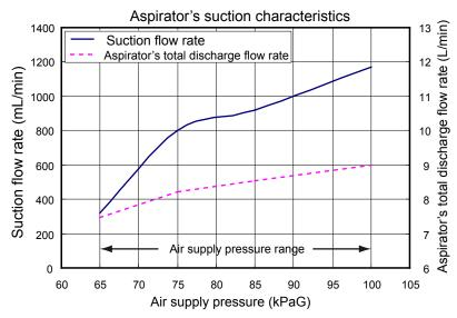
Figure 6.19 Aspirator's Suction Characteristics
