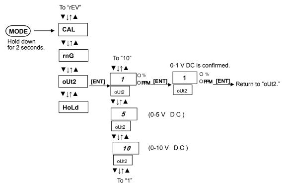
Figure 6.3 Setting Secondary Output "oUt2"
