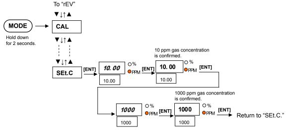
Figure 6.7 Setting Calibration Gas Concentration "SEt.C"
