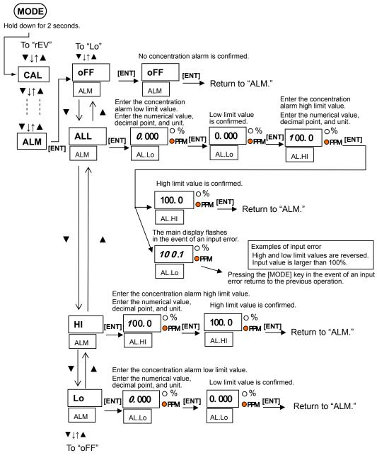
Figure 6.6 Setting Alarm (Oxygen Concentration Alarm) "ALM"
