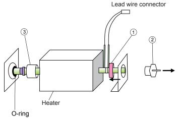
(9) Pull out the holding plate 4, remove the ring 1, and pull the sensor out of the heater straightforward.
