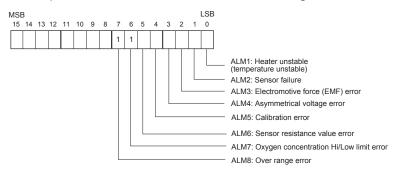
Figure 6.17 Configuration of Alarm Data (00C0)
