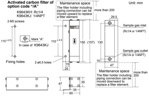
Figure 3.3 Mounting Activated Carbon Filter
