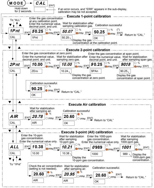
Note: If an error occurs during calibration, that calibration may become invalid. With respect to the action in the event of an error, see Section 7.2.
