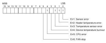
Figure 6.16 Configuration of Error Data (0017)
