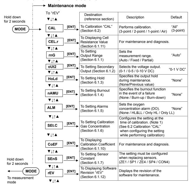
Note 1: When "Air" is selected in Calibration "Cal," the "SEt.C" menu is not displayed.
