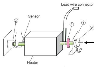
(5) Rotate and tighten the ring ① into the joint ②. Secure the holding plate ④ with two screws (7).
