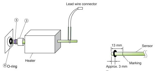
(3) Insert the sensor into the connector and tighten the nut ③ firmly with fingers. At this point, make sure that the lead wire of the sensor is located in the upper right position.
