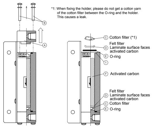
Figure 7.4 How to Replace Activated Carbon
