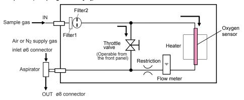
Note: If no suction device [-N] is specified, the aspirator is removed from this diagram.
