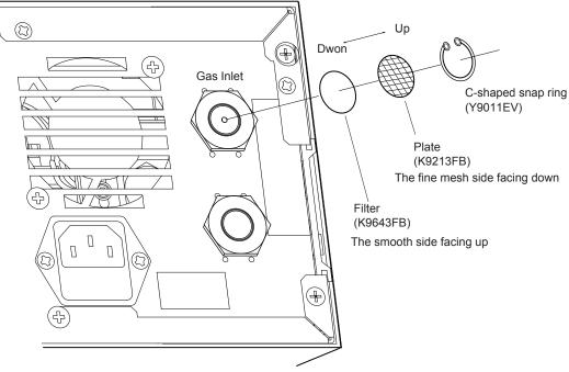
Figure 7.6 How to Replace the Line Filter
