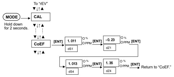
Figure 6.11 Checking Calibration Coefficient "CoEF"
