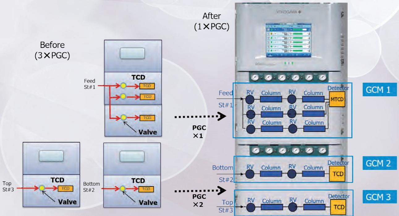
By dividing complex applications into smaller simultaneous measurements, the analyzer complexity as well as analysis time is greatly reduced.
