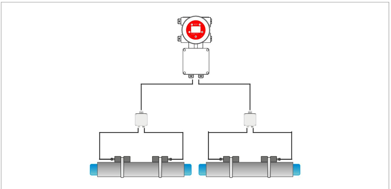
Picture 6: KATflow 170 in a 2-pipe 1-path configuration using optional junction boxes
