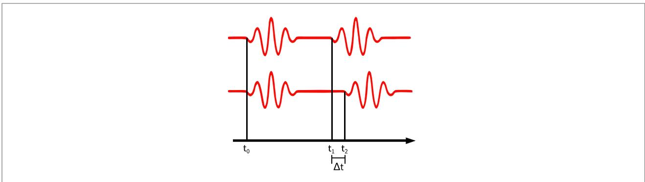
Picture 2: Transit-time measuring principle
