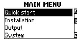
At first power on and the boot sequence, the **Main Menu** is displayed. Use **▲** and **▼** keys to select **Quick Start** and confirm with **ENTER**.
