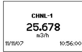
The main measurement unit is displayed when first entering the measurement screen. Press **NEXT** to see up to three units displayed with the main one in the middle. Two further measurement units can be assigned to this screen by going to **Main Menu - Output - Display**.
