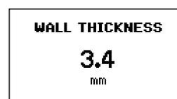
Optional sensor probes to measure pipe wall thickness are available. Ensure the correct pipe material is selected. Connect to the sensor input and select **Start Measurement**.
