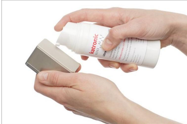
Picture 7: Application of acoustic coupling gel
