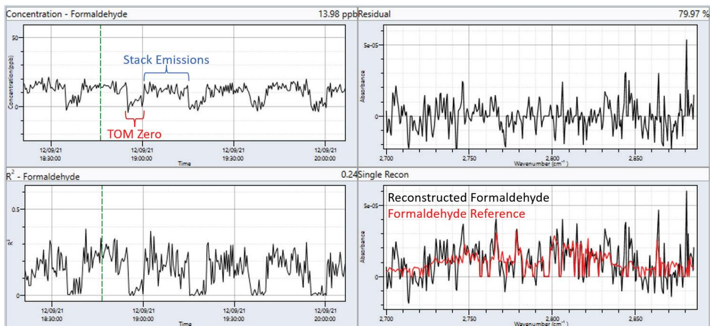
Figure 1: Formaldehyde measurements collected in the field from a natural-gas fired turbine engine.
