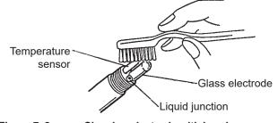
Figure 7.2 Cleaning electrode with brush
