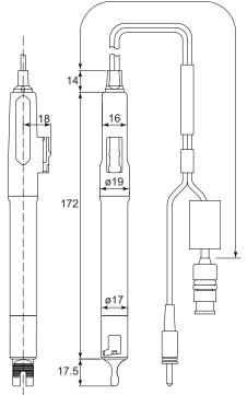
KCI refillable type combination pH sensor Unit: mm PH92SN-21-AA
