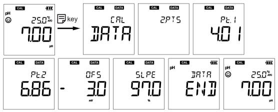
Figure 6.2 Confirmation on calibration data (example for 2 calibration points)
