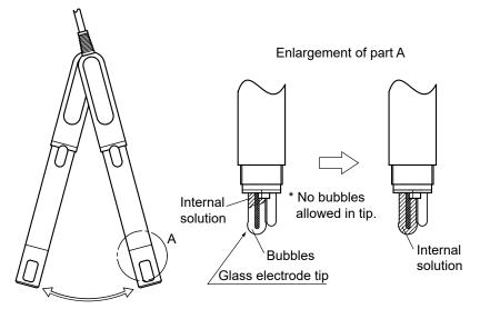
bubbles upward before starting the measurement.
