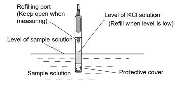
For KCI refillable type sensor, the KCI solution level must be above the measured-solution level.
