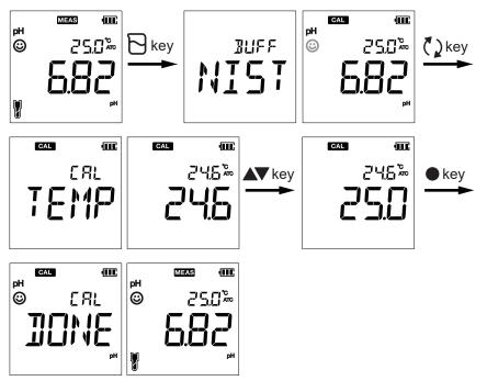
In the manual temperature compensation (MTC) mode, you can manually enter the premeasured temperature of a solution using the above procedure.(page 3-3
