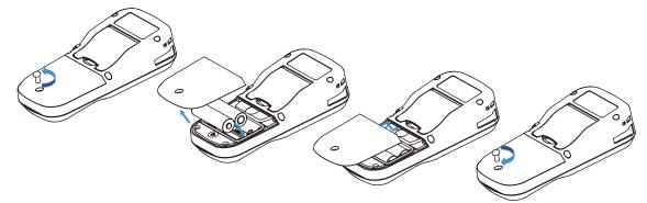
Figure 2.1 Insert battery into the meter
