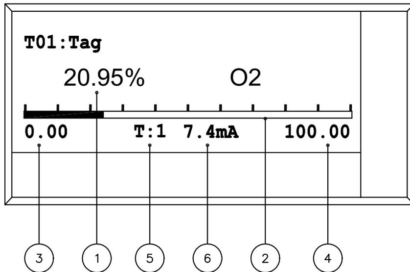
**Figure 6 Measurement format**
