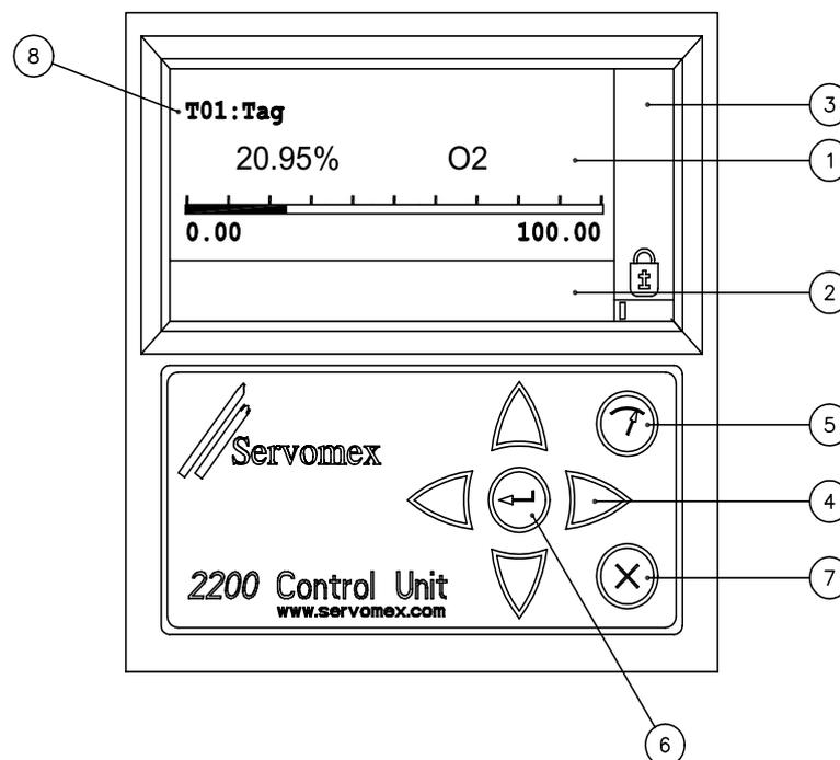
**Figure 1 Control unit display and keypad**
