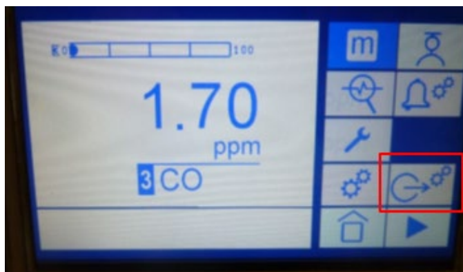
Figure 10-35: Measurement page – Analog Output Settings icon
