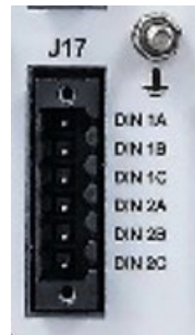
Figure 11-21. Jumper 17 used for Auto-Cal configurations.
