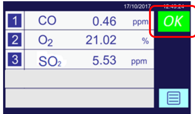
Figure 5-6: Home screen (three gas transducers)
