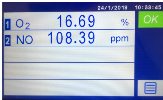
Figure 7-24: NO measurement displayed on Main Screen
