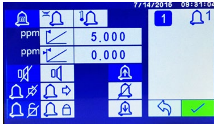
Figure 7-9: Measurement Alarm setup screen for Transducer #1 and Alarm #1
