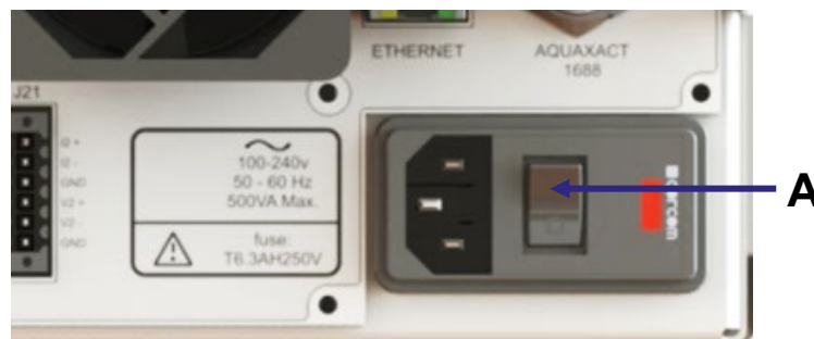
Figure 4-2: On/Off switch on the rear of the analyzer, (A) points to the Power Switch “I” for ON position.
