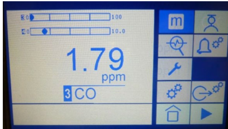
Figure 10-38: Measurement screen showing two analog outputs
