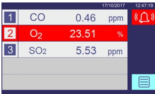
Figure 5-7: Home screen (3 transducer analyzer), showing O 2 alarm
