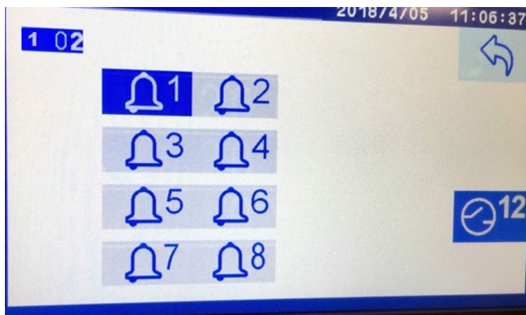
Figure 10-13: Alarm assignment screen for O 2 (Relay #12)
