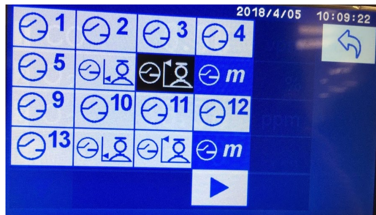
Figure 10-17: Manual relay over-ride of Relay #7 (with Auto-Cal ON)
