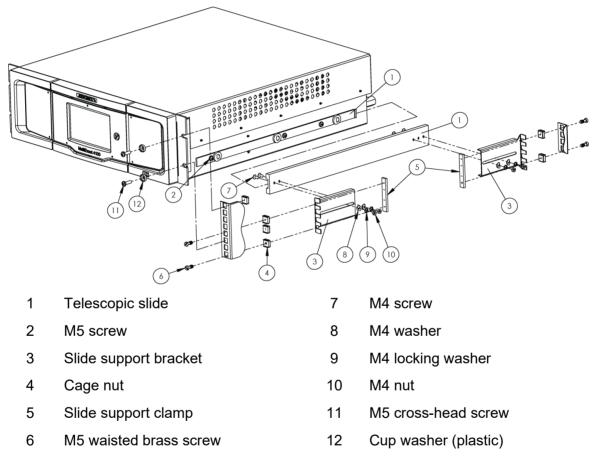
Figure 3-2: Sliding rack installation (M indicates metric value in mm)
