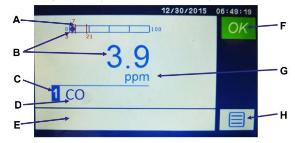
The Home screen (Figure 4-6) displays the current measurement and system status.
