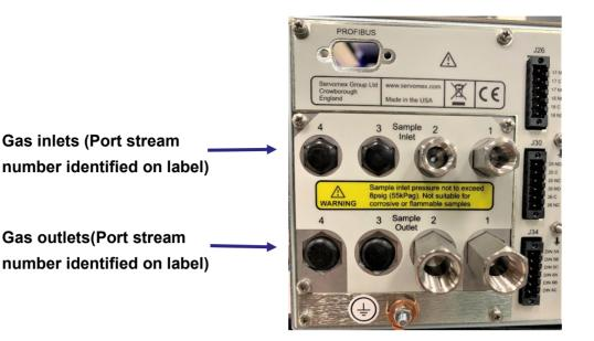
Figure 3-1: Gas inlets and outlets on rear of the analyzer
