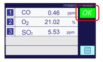
Figure 4-8: Home screen (three gas transducers)
