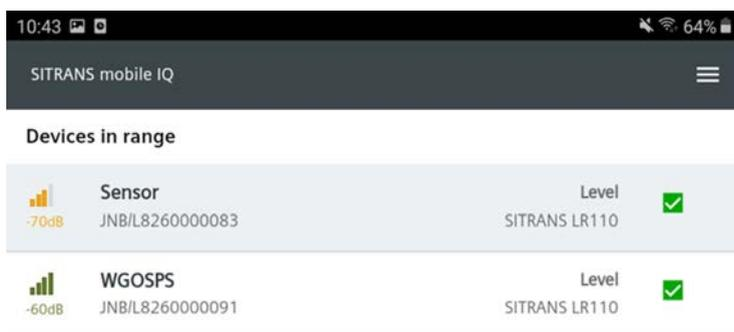
3. Click on the device you wish to connect to. On first connection, a PIN code shipped with the device needs to be entered (see *Device Bluetooth and Parameter Access Codes* sheet). Following successful PIN entry, the device cockpit will be shown.
