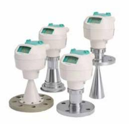
SITRANS LR250 is a 2-wire, 25 GHz pulse radar level transmitter for continuous monitoring of liquids and slurries in storage and process vessels including high temperature and pressure, to a range of 20 m (66 ft).
