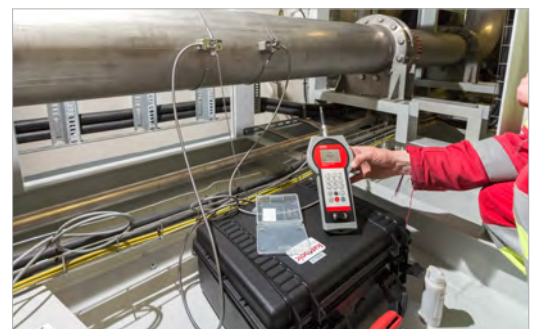
Measurement setup of a portable KATflow 200 on offshore converter platform Helwin alpha.
