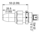
Figure D-1 Dimension drawing SITRANS AW050 Bluetooth adapter, dimensions in mm (inch)
