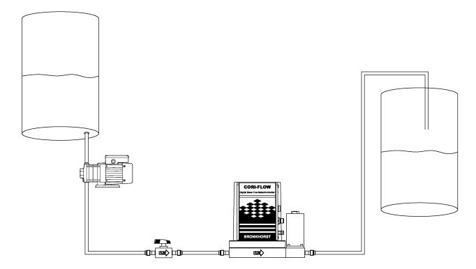
Install the sensor up side down in horizontal position for low flow (< 1000gr/h Full Scale) liquid measurement (see the following figure) and horizontal straight up for higher liquid flows and gas measurement.
