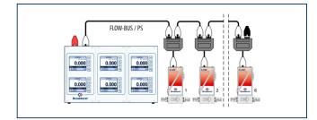
Alternatively only one display can be used to readout these instrument sequentially; model key for this option is E-8101-R-10-00-00
