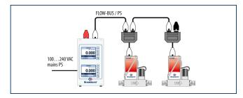
Below you will find a FLOW-BUS set-up with 6 Mass Flow Meters. The model key for this example is E-8101-R-20-20-20
