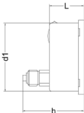
type D (Ø 63 mm, without blow-out back)
