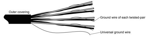
Removing the metallic shield foil from each twisted-pair and the orange wire
