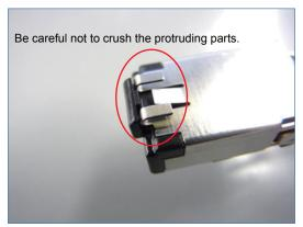
Crimping the cover to the connector body
