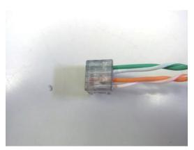
Inserting the cable wires into the connector cover
