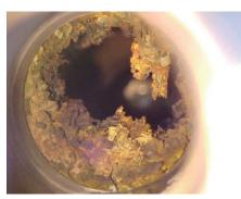
Figure 10.2 Example of deposits in the opening
