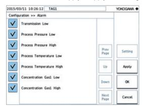
(3) Change the threshold values of each warning. In the following example, to set the threshold value of the transmission low limit alarm, select "Transmission Low," and tap Setting on the right side.
