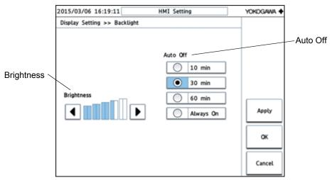
Figure 8.22 YH8000 backlight configuration screen
