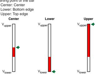
Vupper: Span upper limit (or scale upper limit) Vlower: Span lower limit (or scale lower limit) : Starting point of the bar
