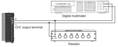
Wiring for current measurement
