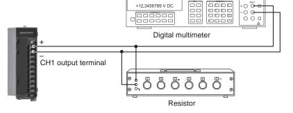
Wiring for current measurement
