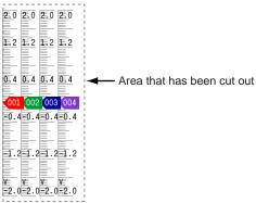
**3** To align the scale position to the positions where the value indicator marks will appear, create guidelines. The lines marked in red on the scale are the guidelines. Erase everything except for the lines marked in red. This image will be used as the base of the scale image.
