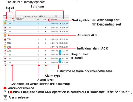
Alarm output release (when alarm ACK is performed)
