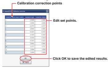
For details on calibration correction, see page 1-53 in section 1.2.4, "Setting Calibration Correction (Linearizer approximation, linearizer bias, Correction Factor 1 (Release number 3 and later))"
