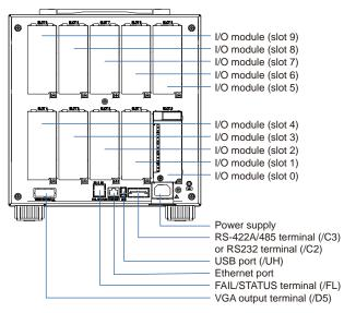
Precautions to Be Taken While Wiring With a screw terminal, we recommend that you use a crimp-on lug with an insulation sleeve (M4 for power supply wiring, M3 for signal wiring).
