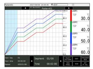
Program screen display: Program operation status display screen: displays the program operating status and the current PV simultaneously (GX/GP only) Number of display loops: 20 max. Number of screens: 1 Display update interval: Digital display area: 500 ms fixed Trend display area: according to the trend interval
