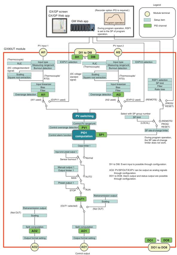
This function can be used when a PID Control Module is installed in GX/GP main unit, expandable I/O, GM main unit, or sub unit.
