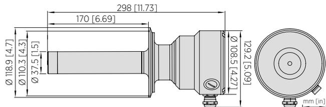
Dimensions of PR53AP Sanitary 4", depth 170 mm
