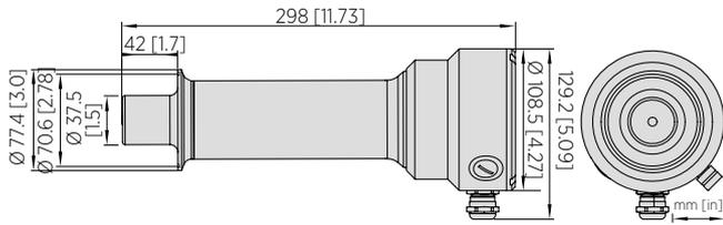
Dimensions of PR53AP Sanitary 2.5", depth 42 mm
