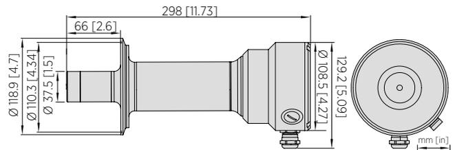
Dimensions of PR53AP Sanitary 4", depth 66 mm
