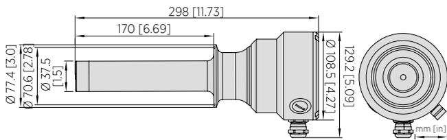
Dimensions of PR53AP Sanitary 2.5", depth 170 mm
