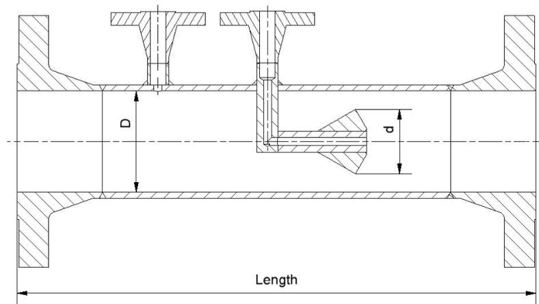
The definition of  $\beta$  for cone meters is different from orifice plates and venturis where  $\beta = d/D$ .
