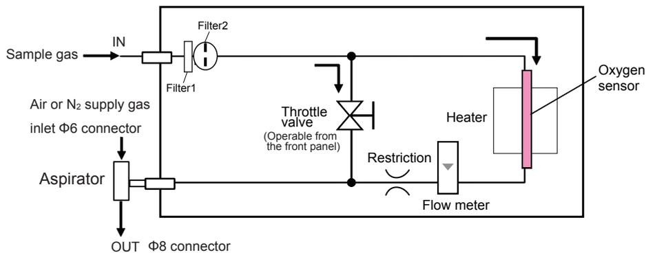
Note: If no suction device [-N] is specified, the aspirator is removed from this diagram.
