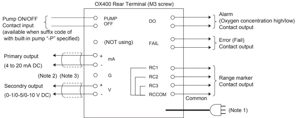
Note 1: Use the earthing contact of power cord to ground to earth.
